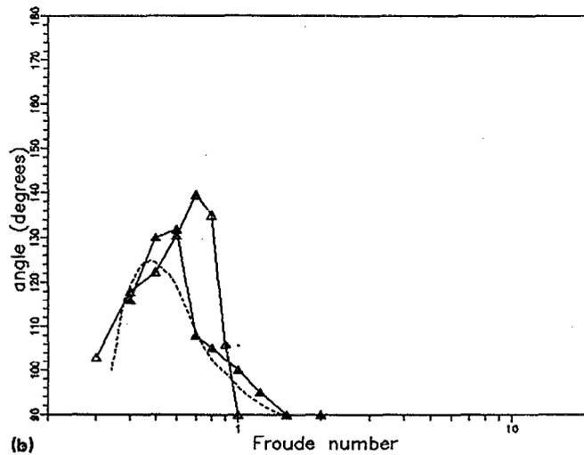
FIG. 2. Variation with  $F$  of the separation points on the sphere. Comparison between fluorescent dye technique ( $\circ$ ,  $\Delta$ ) and shadowgraph technique ( $\bullet$ ,  $\blacktriangle$ ). (a) In the vertical plane for  $Re(1) = 1961$ ; (b) in the horizontal plane for  $Re = 4065$ . ---, Lofquist and Purtell's<sup>11</sup> results.
