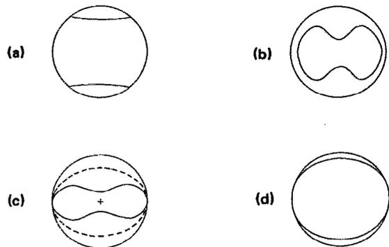
FIG. 5. Shape of the flow separation line on the sphere. (a)  $F = 0.3$ ,  $Re(1) = 1961$ ; (b)  $F = 0.6$ ,  $Re(1) = 1961$ , (c)  $F = 0.9$ , +,  $Re(1) = 324$ , —,  $Re(1) = 1961$ , —,  $Re(1) = 4065$ ; (d)  $F = 1.5$ ,  $Re(1) = 1961$ .
