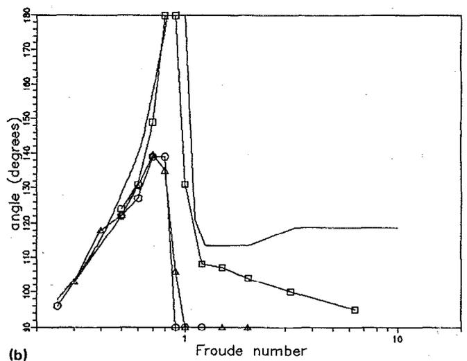
FIG. 3. Variation with  $F$  of the separation points on the sphere. (a) In the vertical plane; (b) in the horizontal plane.  $\square$ ,  $Re(1) = 324$ ;  $\circ$ ,  $Re(1) = 1961$ ;  $\Delta$ ,  $Re(1) = 4065$ ; —, Hanazaki's numerical simulations; ---, Sheppard's theory.
