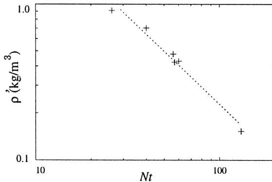
Fig. 14. Decay of the maximum density deviation in the core of a vortex for  $F = 0.4$  at  $y/R \in [0.8; 1.2]$ . The dotted line is the best fit to the experimental data points and exhibits a  $-1.1$  power law.
