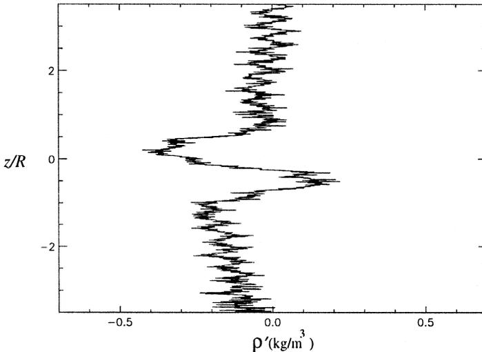
Fig. 16. Vertical profile of  $\rho'(z)$  in the turbulent wake at  $F = 6$ ,  $Nt = 40$  and at  $y/R = 0.8$ .
