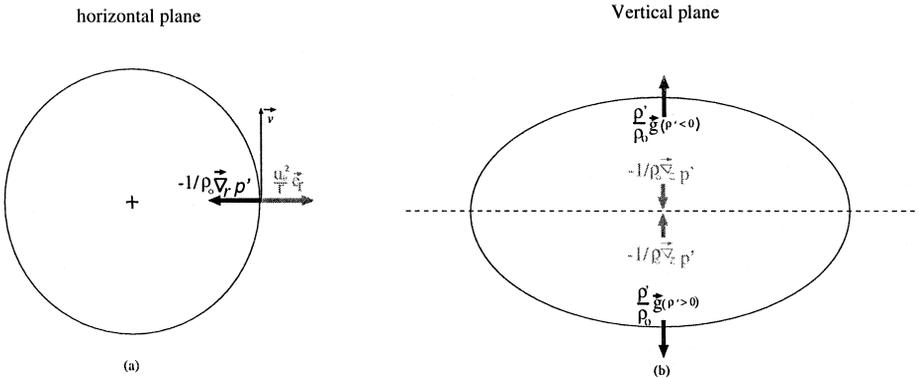
Fig. 3. Schematic view of the balanced state within a vortex structure. (a) Horizontal balance. (b) Vertical balance necessitating lighter fluid in the upper part of the vortex and heavier fluid in the lower part of the vortex.
