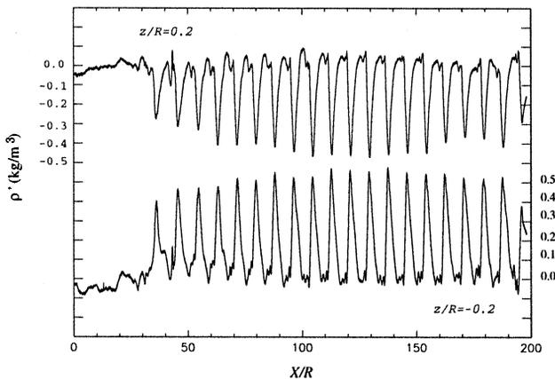
Fig. 8. Two simultaneously acquired density deviation profiles  $[\rho'(X)]$  for  $F = 0.4$ ,  $Nt = 40$ . The two probes are situated above and below the sphere axis at  $x/R = 16$ ,  $y/R = 0.8$  and  $z/R = \pm 0.2$ . The initial portion of the signal corresponds to a region when no vortices are yet present at the probe location.
