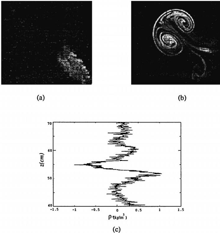
Fig. 17. Measurement of the density anomaly in a turbulent dipole. The dipole is generated by six micro-jets and is visualized using fluorescent dye. (a) Visualisation of the turbulent injected jet, (b) visualization of the dipole at  $Nt = 40$ , (c) vertical  $\rho'(z)$  profile measured at  $Nt = 42$ . The + symbol in (b) shows the position where the vertical density profile was performed.
