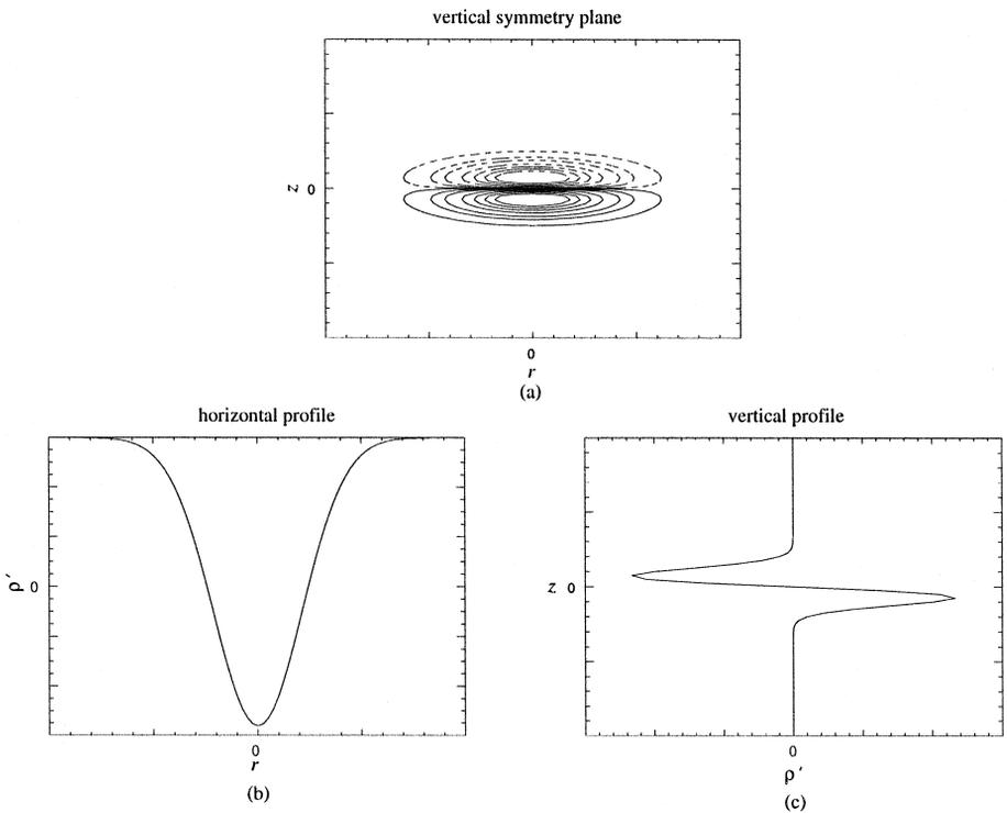
Fig. 4. Density deviation ( $\rho'$ ) of the idealized vortex. (a) Isocontours of  $\rho'(r, z)$  in a vertical symmetry plane (dashed lines, negative values; solid lines, positive values). (b) Horizontal profile of  $\rho'(r)$  at the  $z$ -level coinciding with the minimum density deviation in the upper part of the vortex. (c) Vertical profile of  $\rho'(z)$  through the core of the vortex.
