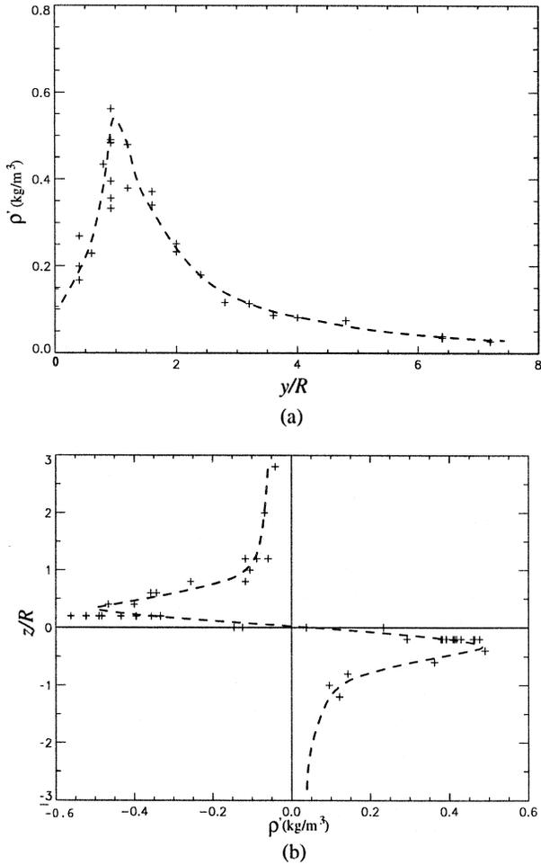
Fig. 9. Mean  $\rho'$  profiles inside a structure at  $F = 0.4$ ,  $Nt = 40$ . (a) Mean horizontal profile of  $\rho'(X)$  realized from a set of profiles at several  $y$ -positions, and for  $x/R = 16$  and  $z/R = 0.2$ . (b) Mean vertical profile of  $\rho'(z)$  realized from a set of profiles at several  $z$ -positions, and for  $x/R = 16$  and  $y/R = 1$ .
