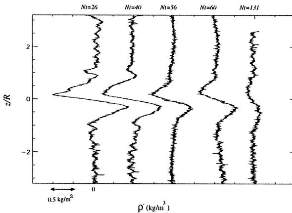
Fig. 13. Temporal evolution of the vertical  $\rho'(z)$  profiles obtained for  $Nt = \{26; 40; 56; 60; 131\}$  at  $F = 0.4$  and at  $y/R \in [0.8; 1.2]$ . Each plot is shifted by  $1 \text{ kg/m}^3$ .
