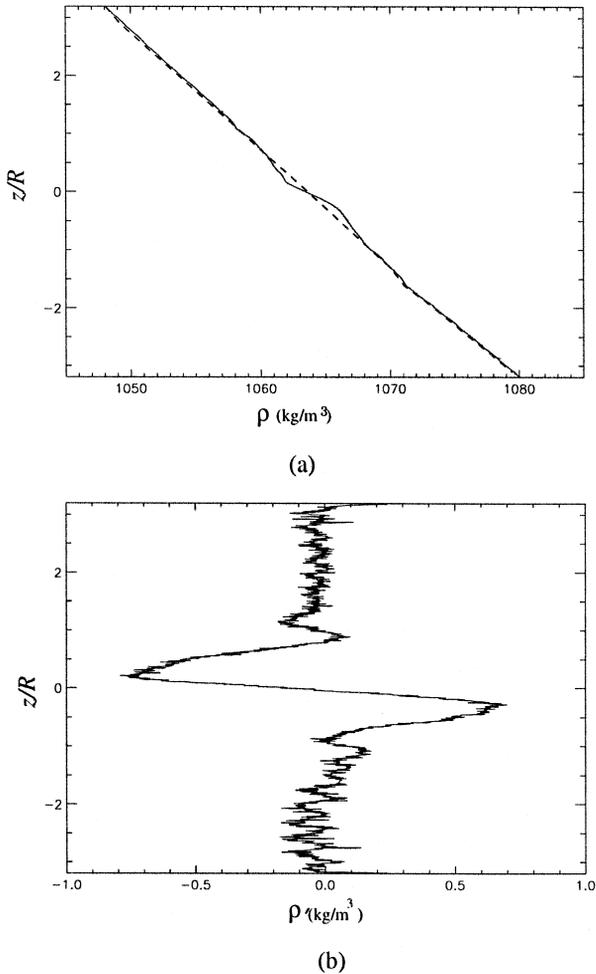
Fig. 10. Vertical density profiles within a structure at  $F = 0.4$ ,  $Nt = 40$ . (a) Superposition of the background stratification measured prior to the tow (dashed line) and the density profile measured in the core of the structure (solid line). (b) Difference of the two signals yielding the density deviation  $[\rho'(z)]$ .
