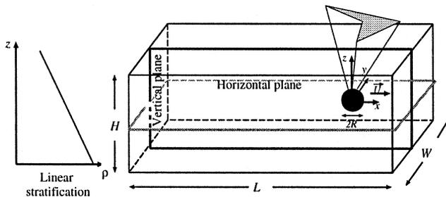
Fig. 1. Schematic diagram of the towing tank. The tank dimensions are  $W = 0.8 \text{ m}$ ,  $H = 0.7 \text{ m}$ ,  $L = 7 \text{ m}$ . The usual linear stratification corresponds to a Brunt–Väisälä frequency close to one.
