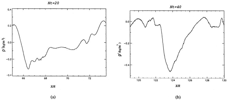
Fig. 12. Zoom of horizontal  $\rho'(X)$  through a single vortex at  $F = 0.4$  and  $z/R = +0.2$ . (a)  $Nt = 20$ , (b)  $Nt = 40$ . Data correspond to those shown in Fig. 11.
