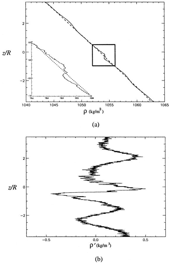
Fig. 15. Vertical profile within the turbulent wake at  $F = 6$ ,  $Nt = 10$  and  $y/R = 1$ . (a) Superposition of the background stratification measured prior to the tow (dashed line) with the density deviation  $\rho'(z)$  measured in the core of the structure (solid line). A zoom of the region of interest is displayed in the left-hand corner of the graph. (b) Difference of the two signals yielding the density deviation  $\rho'(z)$ .
