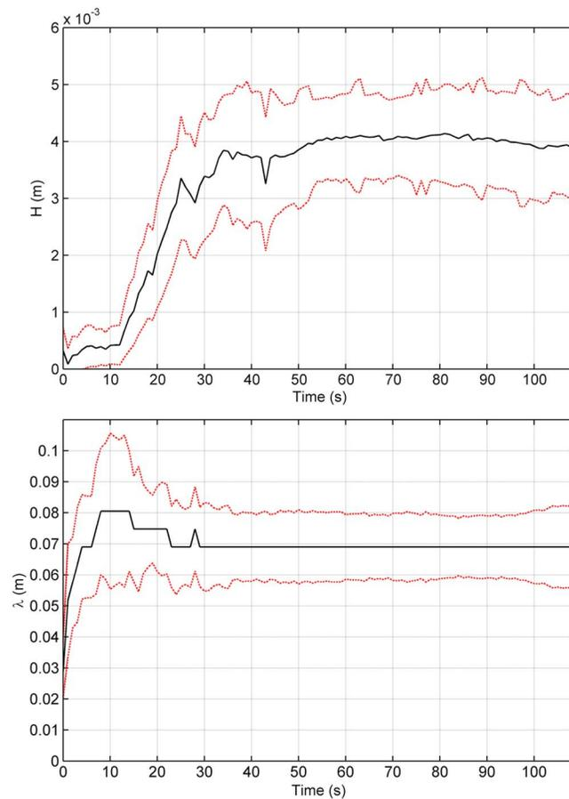
**Figure 4.** Time series of the evolution of the (top) height and of the (bottom) wavelength of the bed perturbations determined by autocorrelation starting with an initially quasi-flat bed. The dashed red lines represent  $H \pm \text{std}$  (Figure 4, top) and  $\lambda \pm \text{std}$  (Figure 4, bottom), with std as the standard deviation.
