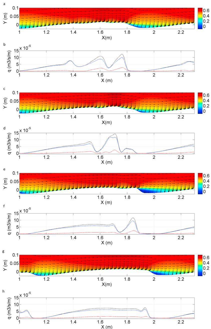
**Figure 14.** Crest degeneration sequence occurring in the zoomed-in subset of Figure 9, with (a, c, e, and g) the velocity field over the bed profile and the bed load (blue), suspended load (red), and total sediment flux (black) at (b)  $t = 2600$  s, (d)  $t = 2640$  s, (f)  $t = 2700$  s, and (h)  $t = 2900$  s.
