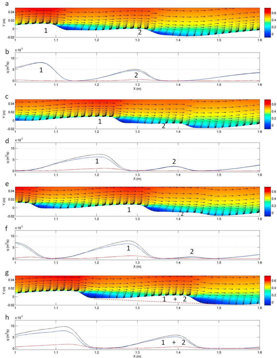
**Figure 7.** Final stage of a merging sequence, with (a, c, e, and g) the velocity field over the bed profile and (b, d, f, and h) the bed load (blue), suspended load (red), and total sediment flux (black) at (b)  $t = 490$  s, (d)  $t = 560$  s, (f)  $t = 600$  s, and (h)  $t = 670$  s.
