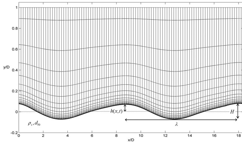
**Figure 2.** Computational grid used over two dunes in the simulation ( $800 \times 40$ ). One of four grid cells is plotted in the  $x$  direction.
