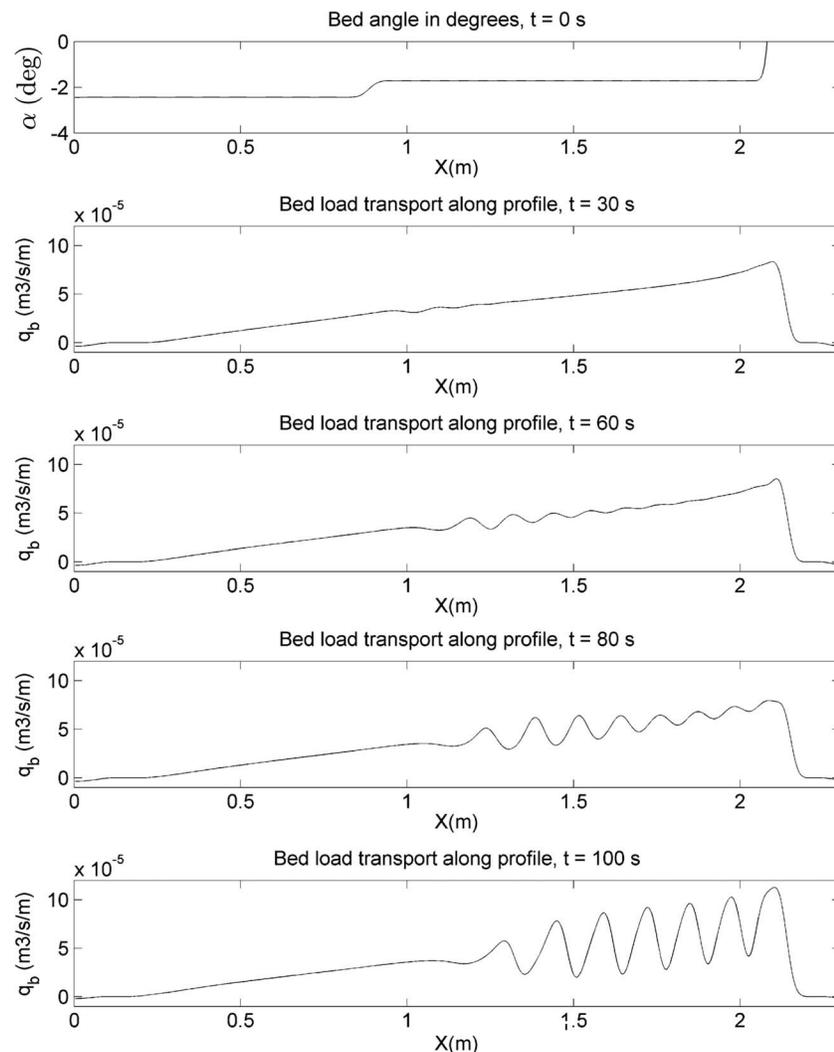
**Figure 11.** Initial bed slope angle ( $\alpha$ ) and bed load transport ( $q_b$ ) along the dune profile from  $t=30$  s to  $t=100$  s for an idealized dune presenting a  $1^\circ$  deflection in its stoss side slope.
