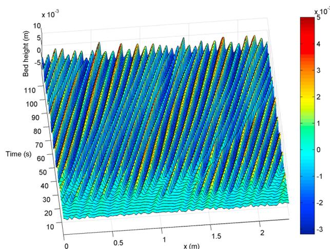
**Figure 3.** Time evolution of a quasi-flat bed in the early stages between  $t=0$  s and  $t=120$  s.
