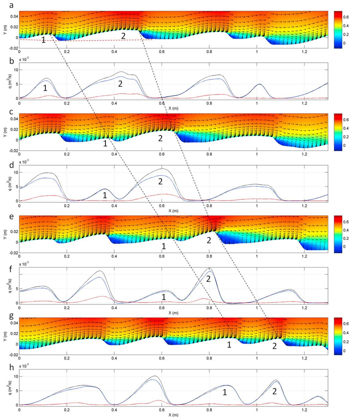
**Figure 6.** First stage of a merging sequence, with (a, c, e, and g) the velocity field over the bed profile and (b, d, f, and h) the bed load (blue), suspended load (red), and total sediment flux (black) at (b)  $t = 100$  s, (d)  $t = 200$  s, (f)  $t = 300$  s, and (h)  $t = 400$  s.
