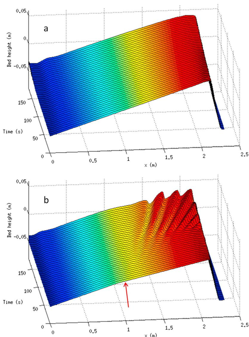
**Figure 10.** (a) Time evolution of an idealized triangular-shaped dune and (b) time evolution of an idealized triangular-shaped dune presenting a deflection of 1° (pointed by a red arrow) in the stoss side slope. The vertical scale is exaggerated 10 times and the red arrow shows the position of the slope deflection.
