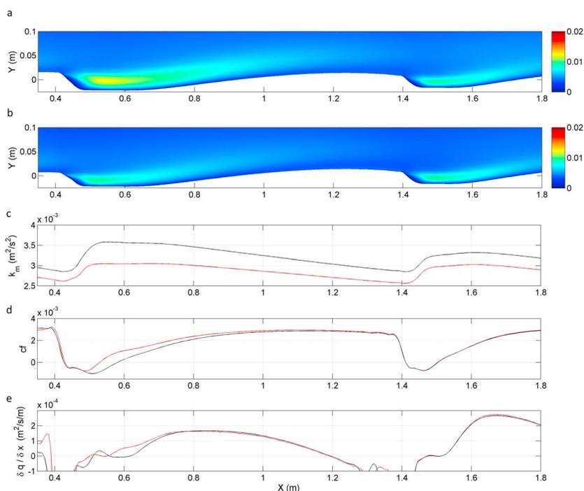
**Figure 12.** (a) Turbulent kinetic energy field  $k$  at  $t = 1850$  s for the baseline simulation (scenario 1) and (b) with a 25% lower upstream dune (scenario 2) with the corresponding spatial evolution of (c) the mean turbulence in the water column,  $k_m$ , (d) the skin friction coefficient  $c_f$ , and (e) the total transport gradient  $\Delta q / \Delta x$  for scenario 1 (black) and scenario 2 (blue).
