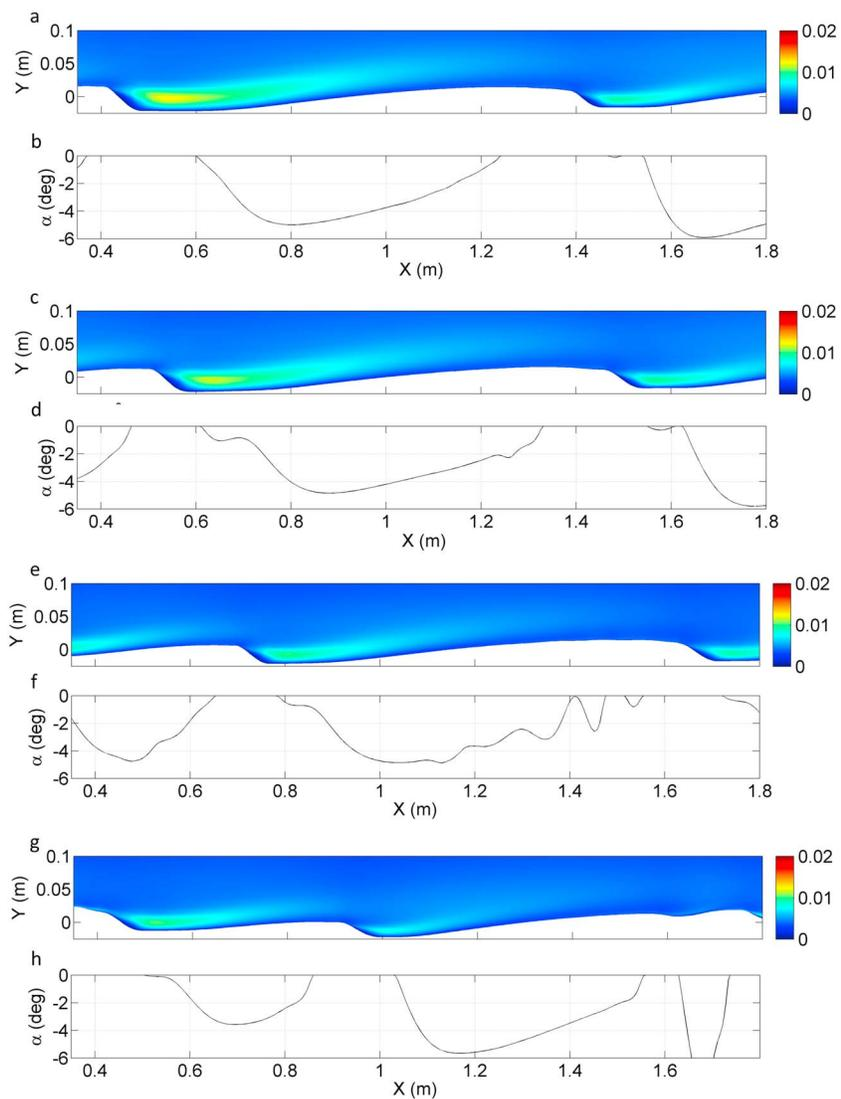
**Figure 13.** Deflection shifting sequence with (a, c, e, and g) the turbulent kinetic energy field,  $k$ , and the bed slope along the bed profile,  $\alpha$ , at (b)  $t=1850$  s, (d)  $t=2000$  s, (f)  $t=2300$  s, and (h)  $t=2650$  s. Higher values at the crest are not shown for a better visualization.
