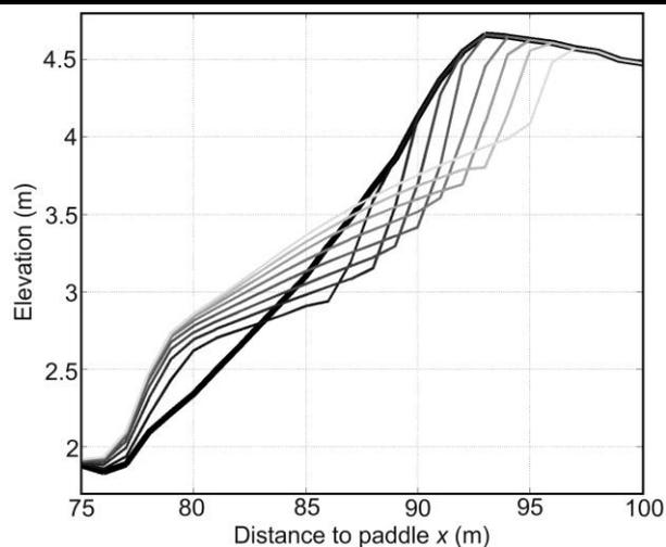
Figure 7. XBeach model results for test series D1 (measured beach profiles for the same sequence as shown in Figure 3).
