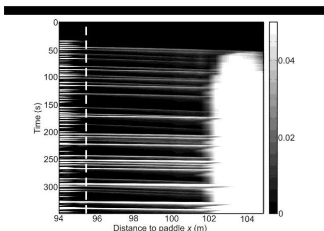
Figure 8. Simulation of overtopping with SURF-GN at the start of test series D1-07. The vertical dotted white line and the colorbar indicates the barrier crest location the height of the water pellicle, respectively.
