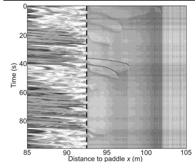
Figure 5. 100-s timestack during D1-07 showing occasional overtopping (two examples are highlighted with the thin dotted black lines at  $t \approx 40$  s). The vertical black dashed line indicates the barrier crest location, as seen by the camera (the actual position is  $x \approx 95.5$  m), that shadows the beach.
