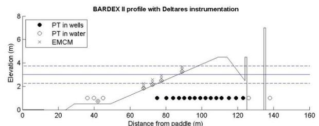
Figure 1. Delta Flume cross-section with barrier profile at the start of the experiment and location of Deltares instrumentation. PT = pressure transducer; EMCM = electromagnetic current meter. Horizontal lines show water levels used.
