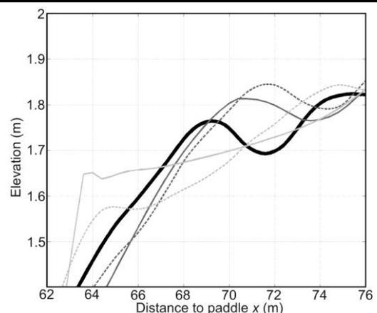
Figure 6. Simulation of beach profile evolution with 1DBeach during test series C2. Zoom at  $62 \text{ m} < x < 76 \text{ m}$ . Initial beach profile (thick black line, ripples are filtered), measured (thin dotted line) and simulated (thin solid line) beach profile at the end of the slow onshore migration (dark gray) and at the end of the rapid offshore migration (light gray).
