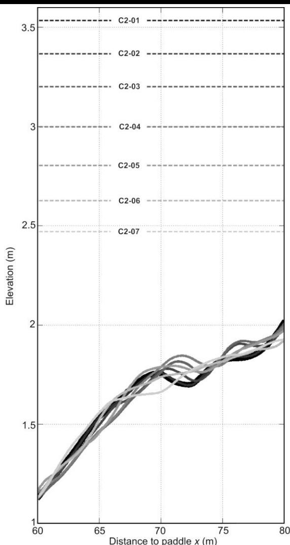
Figure 2. Test series C2 with time-varying sea level (dashed lines) and zoom of the measured beach profiles (ripples are filtered) at  $60 \text{ m} < x < 80 \text{ m}$ . Time evolution is shown from black to light grey. From C2-01 to C2-04 the sandbar initially located at  $x \approx 70 \text{ m}$  slowly migrates onshore and further rapidly migrates offshore from C2-05 to C2-07 as the sea level drops.
