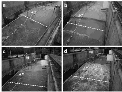
Figure 4. Photo sequence showing drastic beachface shape changes during test series D1 with rising sea level. (a) Gently sloping beach face turning into (b) an erosion scarp of about 20 cm high that is subsequently (c) flattened through increasing overtopping and (d) lowering of the crest through overwash processes. Note that in panel (d) the barrier becomes saturated. In all panels, the dashed white line indicates the initial barrier crest position.
