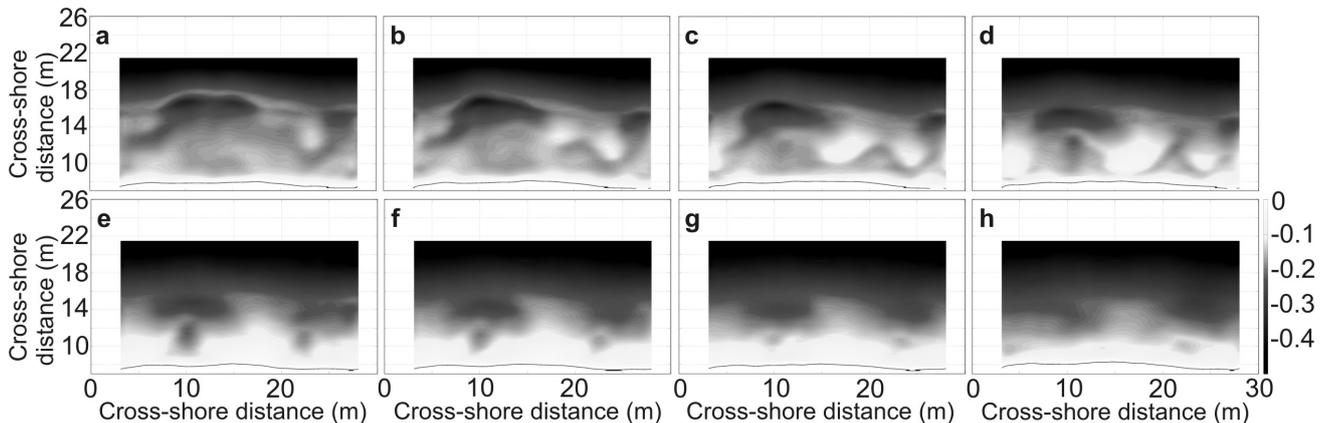
Figure 2. Beach morphologies surveyed with millimeter accuracy corresponding to the eight situations (from runs a to h) described in this paper. Colorbar indicates seabed elevation in meters.
