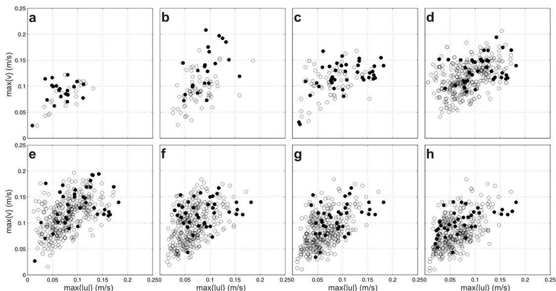
Figure 5. For every drifter, maximum offshore-directed (alongshore) velocity  $\max\{v\}$  the drifter experienced within the rip current circulation during the single last rotation. For the 8 situations from video runs a to h, drifters subsequently exiting the surf zone compartment (1.25Xs) are black circles and those being subsequently retained in the rip current circulations are white circles.
