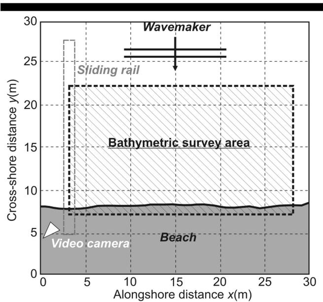
Figure 1. Schematic set-up for the laboratory experiment with delimitations of the bathymetric survey area (dashed box) and location of the video camera that was used to track the drifters.
