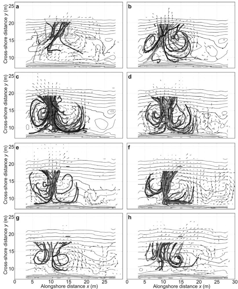
Figure 4. Computed mean flow patterns computed in *Castelle et al. (2010)* with the local bottom morphology contoured in the background for the eight situations from video runs a to h. The pathlines (thick grey lines) of all the drifters exiting the surfzone compartment are superimposed.
