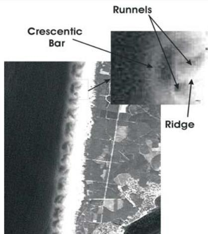
Figure 1. SPOT image of Truc Vert Beach, SPOT XS1, 15/05/01@CNES -DGO- UMR EPOC; Nearshore crescentic bar associated with a half-wavelength ridge and runnel system and intermediate crescentic system
