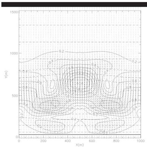
Figure 7. Wave-induced current vector plot over a crescentic bar. Offshore wave conditions:  $H_s=4\text{m}$ ,  $T=6.5\text{s}$ ,  $\theta=0^\circ$ ,  $\eta=4\text{m}$ . Dashed line: bathymetry; Black line: iso-value of wave-induced currents ( $\text{m}\cdot\text{s}^{-1}$ ).
