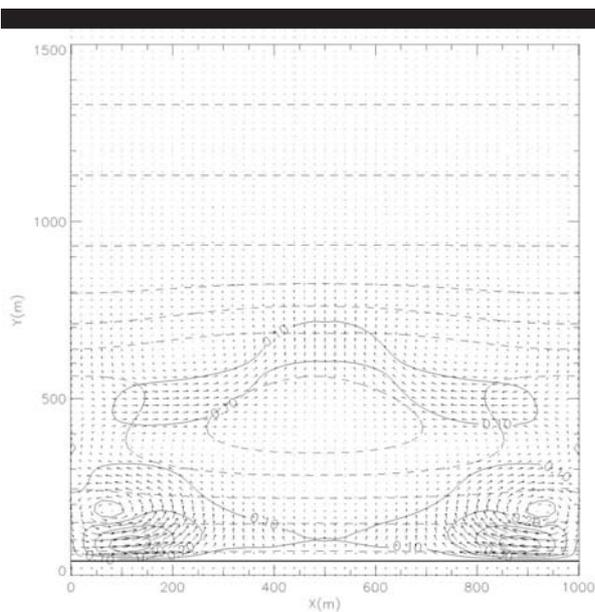
Figure 6. Wave-induced current vector plot over a crescentic bar. Offshore wave conditions:  $H_s=1.36\text{m}$ ,  $T=19\text{s}$ ,  $\theta=0^\circ$ ,  $\eta=4\text{m}$ . Dashed line: bathymetry; Black line: iso-value of wave-induced currents ( $\text{m}\cdot\text{s}^{-1}$ ).
