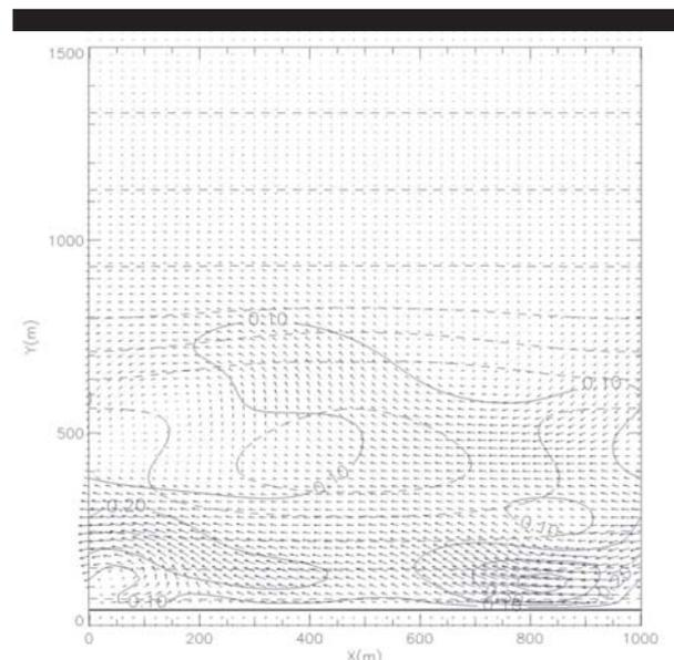
Figure 5. Wave-induced current vector plot over a crescentic bar. Offshore wave conditions:  $H_s=1.36\text{m}$ ,  $T=6.5\text{s}$ ,  $\theta=5^\circ$ ,  $\eta=4\text{m}$ . Dashed line: bathymetry; Black line: iso-value of wave-induced currents ( $\text{m}\cdot\text{s}^{-1}$ ).
