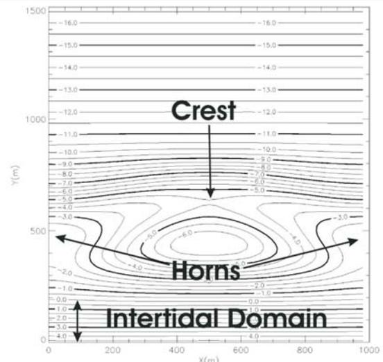
Figure 2. Periodic numerical bathymetry of nearshore crescentic bar, the shoreline is to the bottom.
