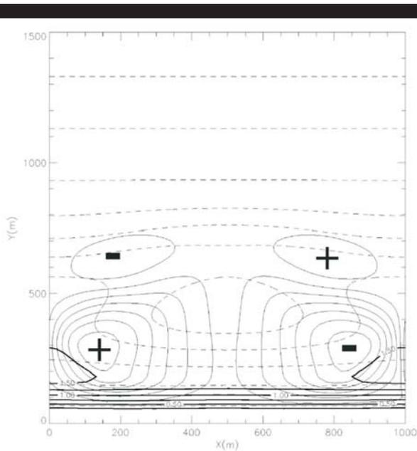
Figure 3. Radiation stress  $S_{xy}$ . Offshore wave conditions:  $H_s=1.36\text{m}$ ,  $T=6.5\text{s}$ ,  $\theta=0^\circ$ ,  $\eta=4\text{m}$ . Dashed lines: bathymetry; Thick lines: iso value of  $H_s$  (m). Black lines: iso value of  $S_{xy}$
