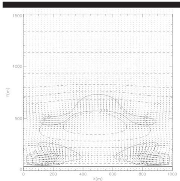
Figure 4. Wave-induced current vector plot over a crescentic bar for the reference offshore wave conditions at high tide:  $H_s=1.36\text{m}$ ,  $T=6.5\text{s}$ ,  $\theta=0^\circ$ ,  $\eta=4\text{m}$ . Dashed line: bathymetry; Black line: iso-value of wave-induced currents ( $\text{m}\cdot\text{s}^{-1}$ ).
