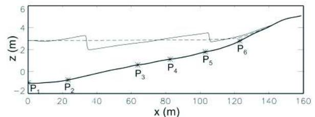
Figure 1. Bottom topography (thick line) measured along one transect at Truc Vert beach on October 18<sup>th</sup> 2001 and locations of pressure sensors (P1-P6). Numerical simulations at high tide ( $t=t_h$ ): instantaneous water surface elevation (solid line), 10 min-averaged water surface elevation (dashed line).
