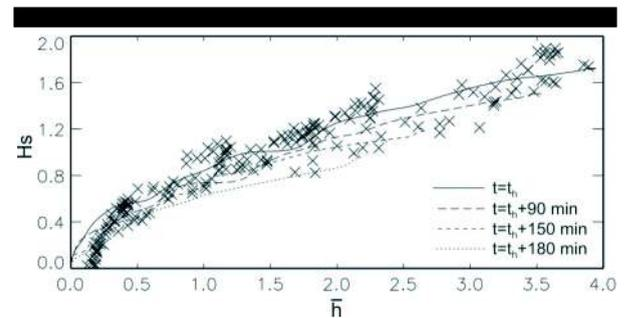
Figure 7. Observed (X) and predicted (line) significant wave height versus mean water depth. Experimental data correspond to the whole data set ( $t \in [t_i, t_i+203 \text{ min}]$ ).
