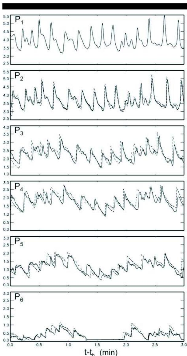
Figure 4. Comparison between observed (solid line) and predicted (dashed line) time series of water depth at sensors P1-6;  $t=t_h$ .
