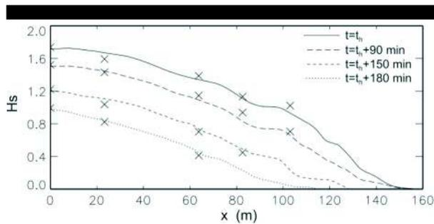
Figure 6. Observed (X) and predicted (line) significant wave height versus cross-shore distance.
