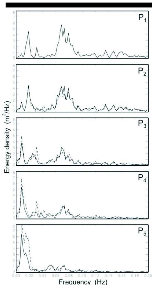
Figure 5. Comparison between observed (solid line) and predicted (dashed line) sea surface elevation density spectra at sensors P1-5;  $t=t_h$ .
