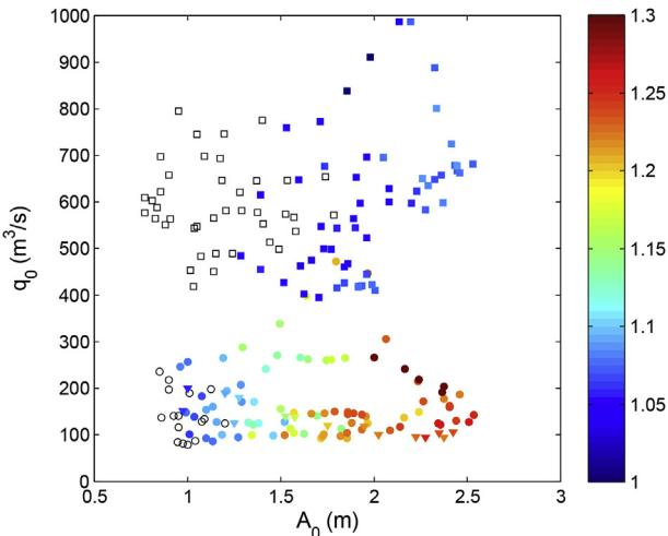
**Fig. 6.** Position of the tides, observed during 3 field campaigns on the Gironde/Garonne estuary, in the plane ( $A_0$ ,  $q_0$ ). Close and open symbols correspond to tidal wave with and without tidal bore respectively; square symbol, TBG1 campaign; circle symbol, TBG2 campaign; triangle symbol, TBG3 campaign; the colormap shows the tidal bore Froude number.
