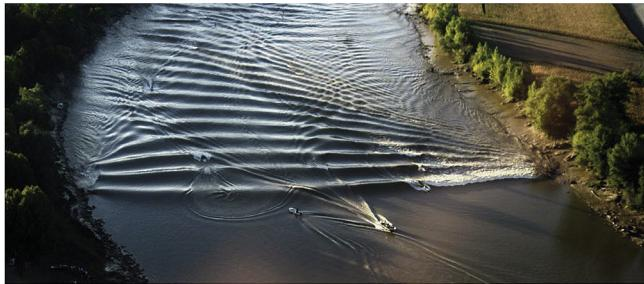
**Fig. 1.** Illustration of a tidal bore propagating in the Garonne River. Aerial photograph taken at Podensac on September 10, 2010. Tidal wave amplitude at the estuary mouth  $A_0 = 2.5$  m and freshwater discharge  $q_0 = 128 \text{ m}^3/\text{s}$ .
