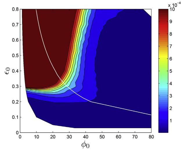
**Fig. 4.** Maximum slope of the tidal wave at  $x = 3L_{bo}$ ; the colormap is limited to slope values below  $10^{-3}$ , a value above where we consider TB occurring; each point in the plane ( $\phi_0$ ,  $\varepsilon_0$ ) represents the numerical tidal wave solution for an idealized convergent estuary of constant convergent parameter:  $\delta_0 = 2$ ; this figure relies on 225 numerical simulations (Arpaia et al. (2015)); white line, zero-amplification curve.
